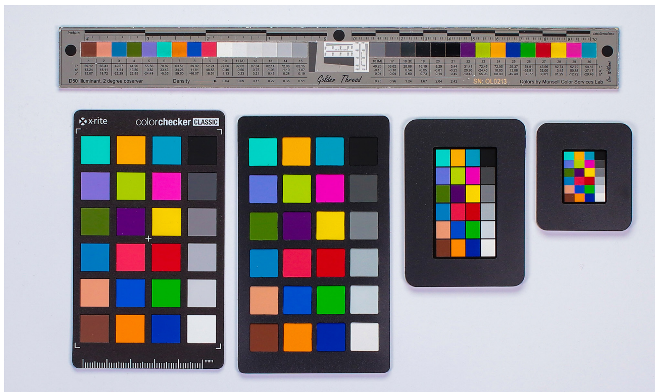
Figure 1. Tested reference charts: A – Golden Thread Object Level; B – X-Rite ColorChecker Classic Mini; C – Charttu 24 Mini; D – Charttu 24 Micro; E – Charttu 24 Nano.
